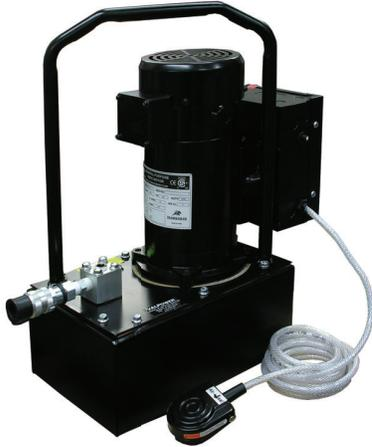
**NOTE:** These instructions cover all 'Automatic Return' style pumps. Some units may have different specifications than others and may have additional items. Electric models with standard manifold block are illustrated.
