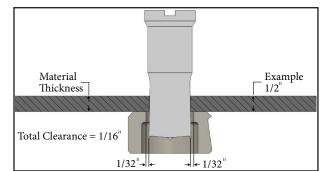
NOTE: The thickness of the material should not exceed the punch diameter.
